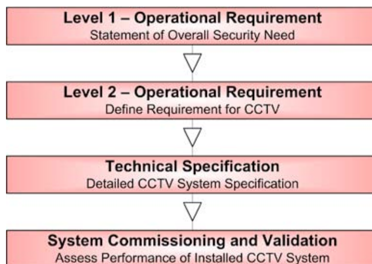
Figure 1: Key stages in specifying a CCTV system
