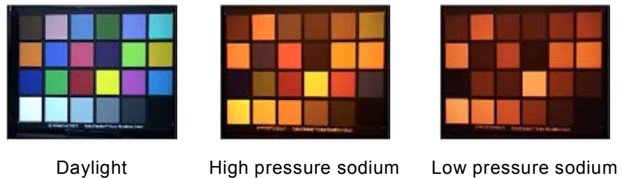
Figure 7: Macbeth Colour Checker Chart® under different light sources, showing loss of colour information
